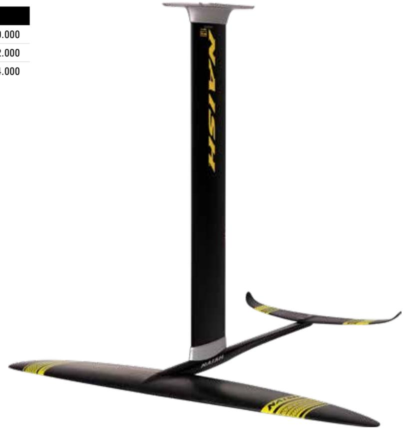
To make the S25 complete foil Naish's best yet, each component has been completely redesigned with an emphasis on making them ultra-lightweight and strong. The mast is a new design that is 25% lighter while improving bending resistance and torsional strength. The mast features a new bonding system to the board mount as well as the fuselage connection resulting in a sealed and more direct board connection system.
